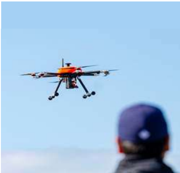
Shown flying is OBSIDIAN, which uses counter-drone technology, specifically designed to detect, identify and track small / micro drones.
