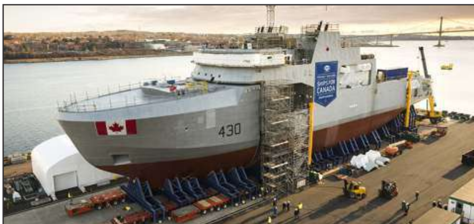
The final mega block was joined to the first two mega blocks, to make up the entire vessel.
