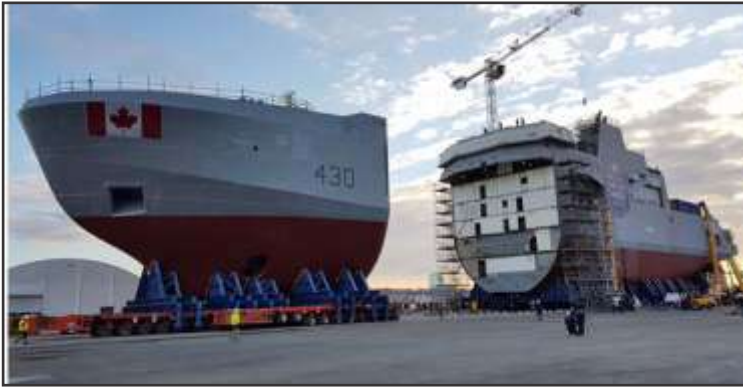
Joining of mega blocks
